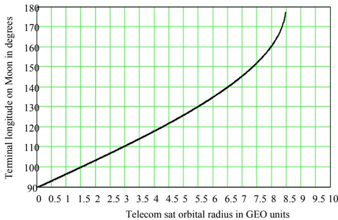
**Figure 4** Terminal longitude  $\lambda$  (vertical axis) on the Moon Farside versus the telecom satellites orbital radius  $R$  around the Earth (horizontal axis) expressed in units of the Earth's geostationary radius (42241.096 km).
