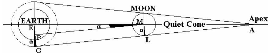
**Figure 3** The simple geometry defining the “Terminal Longitude,  $\lambda$ ” on the Farside of the Moon, where radio waves emitted by telecom satellites circling the Earth at a radius  $R$  are grazing the Moon surface.
